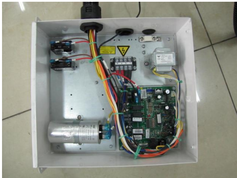
Electric box internal view
